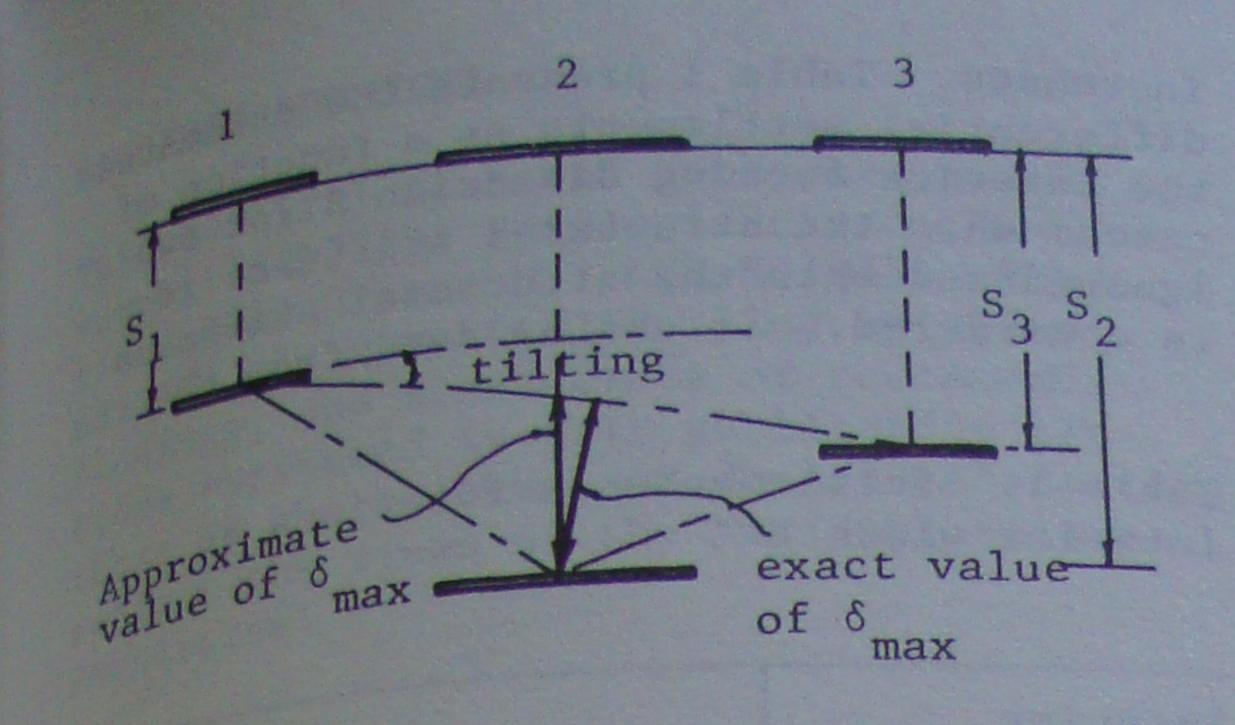
Figure 2. Definition of the maximum differential settlement,  $\delta_{\text{max}}$
