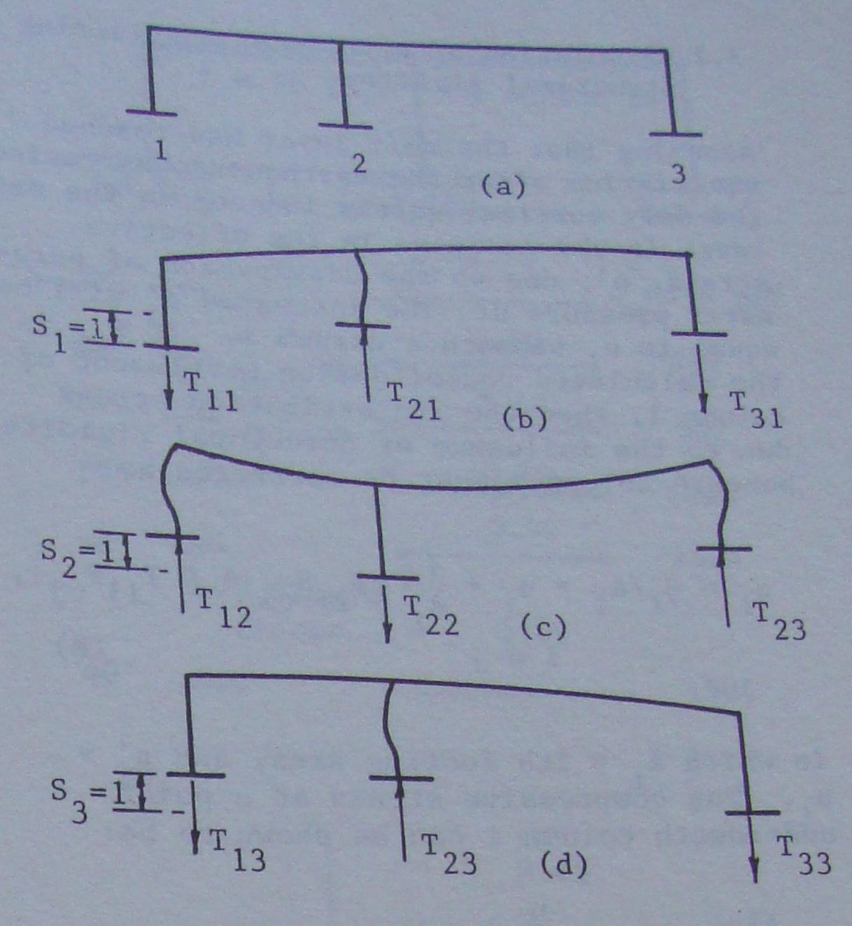
Figure 1. Load transfer coefficients for a two-bay one-story frame
