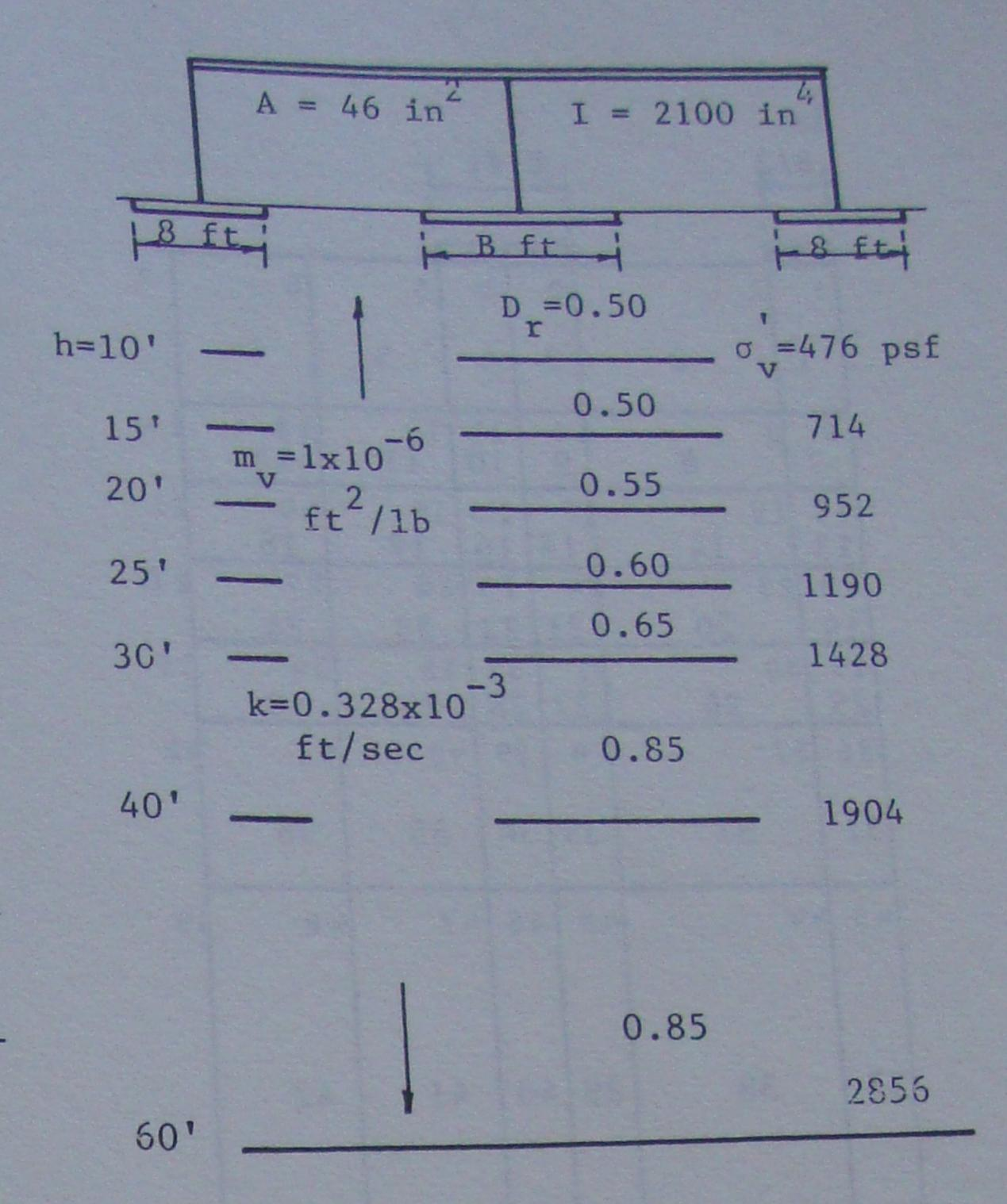
Figure 3. Spread footings foundation and soil strata
